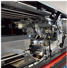
The system can optionally be factory fitted with an automatic adjustment device. This allows the changeover to be reduced to a few simple steps by the operator. This very short changeover time and rapid availability for new jobs is a major strength of the Kern 1600.
